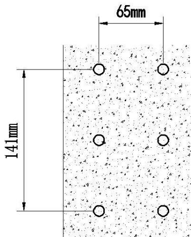
2. Connect and fix the speaker to be mounted with the hanger, and then lock it on the expansion bolts previously installed. According to needs, adjust the pitch and horizontal angle of the speaker; (Pull out and insert the angle adjustment bolt from B to adjust the pitch angle of the speaker. Remove the rubber nut cap from A, loosen and tighten the M8 self-locking nut appropriately, and turn the speaker left and right to adjust the horizontal angle of the speaker.)
