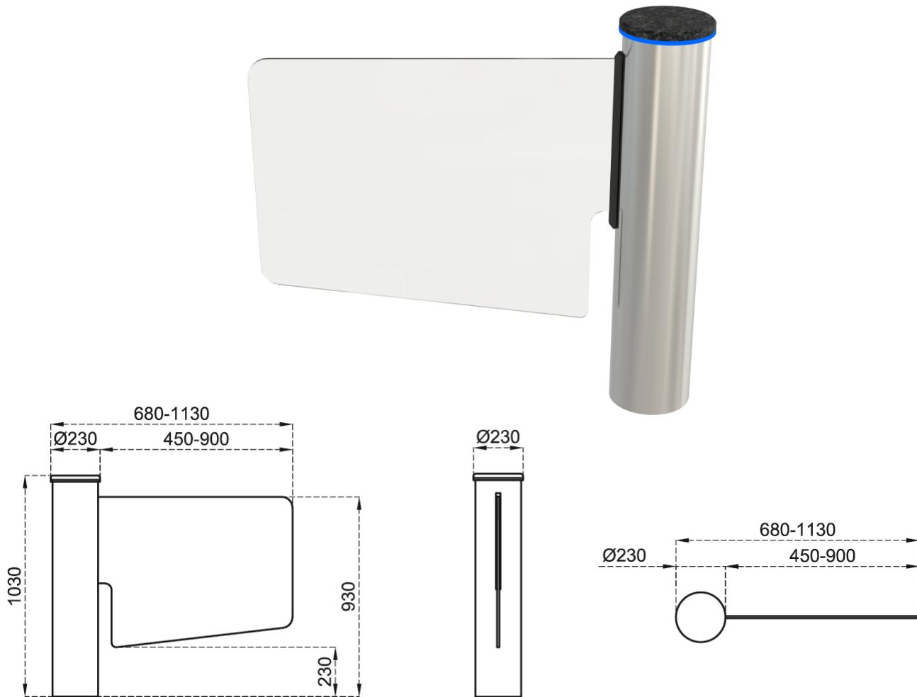
**Power Requirements :** 110/220-240V. 60/50Hz. AC (%±10) 24V.DC at standby ~2W.max. ~65W.
